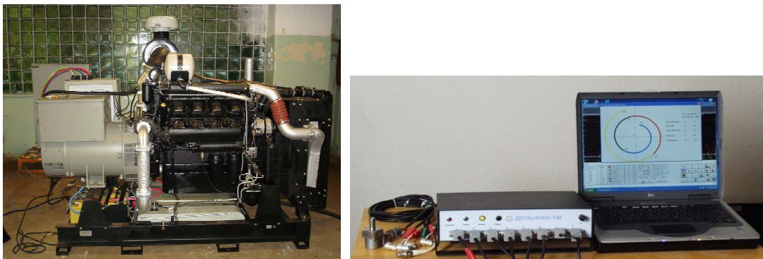
Fig. 1. Experimental installation and stand of vibroacoustic diagnostics
